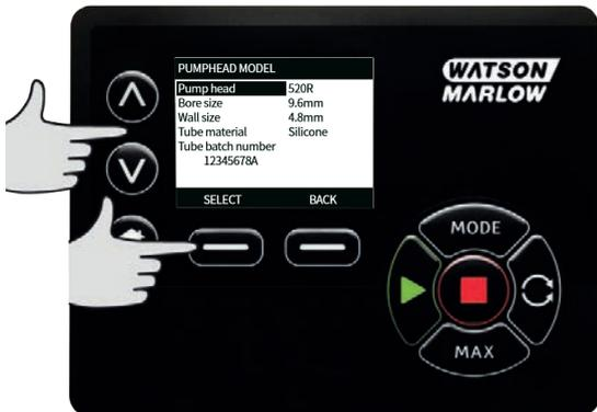
Use the ^ / v keys to move the selection bar over the required pumphead type and press **SELECT**.
