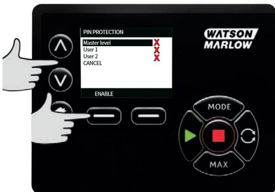
To define a four digit Master PIN, use the  $\wedge$  /  $\vee$  keys to select each digit from 0-9. Once you have the required digit press the **NEXT DIGIT** key. After selecting the fourth digit press **ENTER**.
