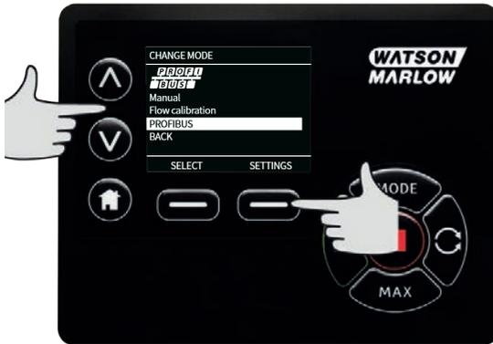
Use the  $\wedge$  and  $\vee$  keys to alter the station address, in the range from 1 to 125 (126 is the default station address). Press **FINISH** to set the station address, or **NEXT** to enable/disable PROFIBUS communication.
