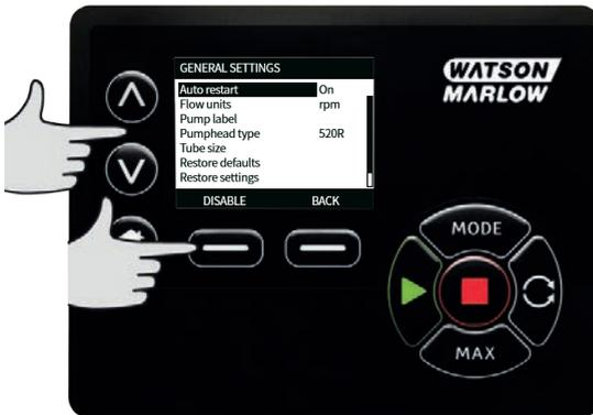
Use the ^ / v keys to move the selection bar over **Pumphead** and press **SELECT**.
