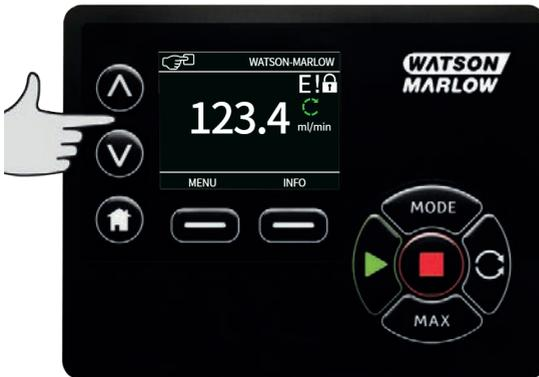
Using the  $\wedge$  and  $\vee$  keys will increase or decrease the flow rate.
