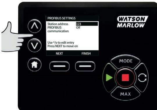
Use the  $\wedge$  and  $\vee$  keys to enable or disable PROFIBUS communication and press **FINISH**.
