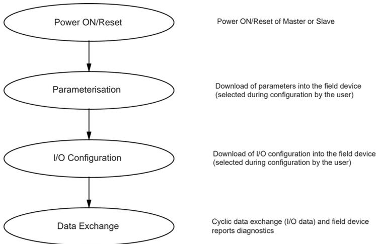
If data exchange is lost at any time, the following Bus Error screen will be displayed. The first red dot corresponds to the stage at which the error occurred and subsequent stages will indicate a red dot because the communication sequence halted before this point.
