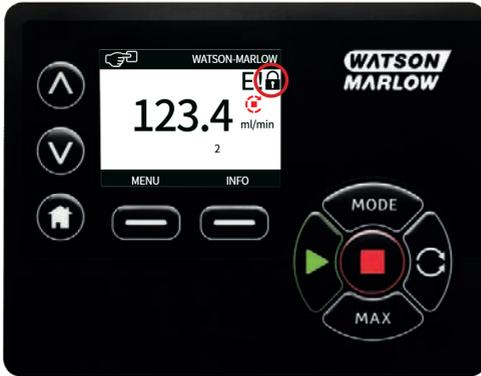
Note that the STOP key will always work whether the keypad is locked or not.
