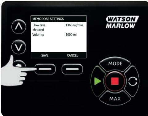
When MemoDose SETTINGS are complete the following screen is displayed; press **MEMODOSE** to start in MemoDose Mode or **BACK** to return to MemoDose settings.
