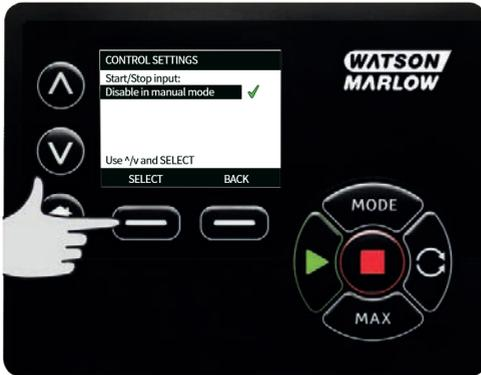
Use the  $\wedge$   $\vee$  keys and press **SELECT** to choose the logic state of the chosen input for your connected control hardware.
