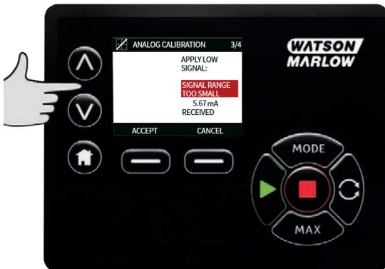
ACCEPT appears when low mA signal is within tolerance limits. Press **ACCEPT** to accept the low signal input or **CANCEL** to return to the previous screen.
