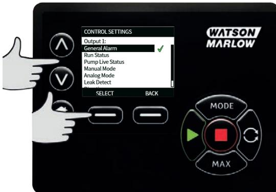
Use the  $\wedge$  /  $\vee$  keys and press **SELECT** to choose the logic state of the chosen output.
