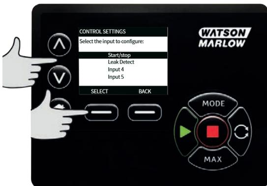
Use the  $\wedge$  /  $\vee$  keys and press **SELECT** to choose the logic state of the chosen input.
