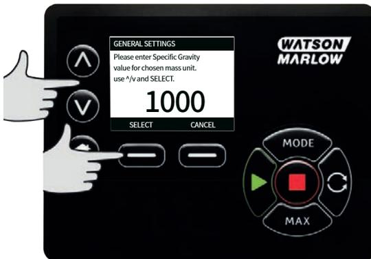
Use the  $\wedge$  /  $\vee$  keys to enter the value of the specific gravity, and press **SELECT**.
