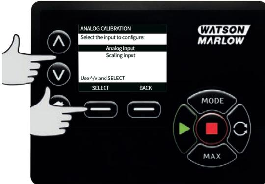
Select the input signal type using the  $\wedge$   $\vee$  keys and press **SELECT**.
