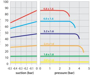
Flows obtained pumping water at 100rpm CCW-rotation
