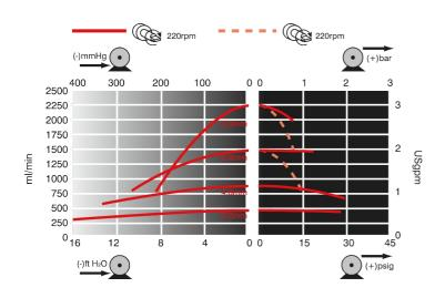
Maximum duty pressure with 6.4mm and 8.0mm bore tube is 1bar. Maximum duty pressure with other tube bore sizes is 2bar.
