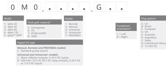
\* The pumphead side location is required when ordering. The left/right perspective assumes the user is looking at the front of the pump. The pump in the dimensions diagram is considered a pumphead located to the left.
