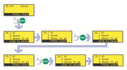
If the batch is set to perform one dose, as in the example shown here, the pump stops when that dose has been dispensed and waits for a further press on the **START** key. As each dose is dispensed, the display increments, recording the number of doses dispensed so far.
