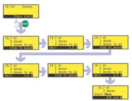
If the batch is set to perform more than one dose with a set interval between doses, the pump operates until all the batch's doses have been dispensed. The display decrements as each dose is dispensed, showing the number of doses still to be dispensed. During the intervals between doses - 3 seconds in the example shown - the time elapsing is counted down to show how much time is left before the next dose will start.
