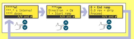
To move from one screen to subsequent screens, repeatedly press DOWN. Each item is highlighted in turn until the last item on the screen is highlighted. A further press on the DOWN key displays the next screen of the menu, with the first item highlighted.
