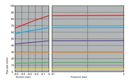
Marprene tubing, 1.6mm wall, 100 rpm, CCW rotation.
