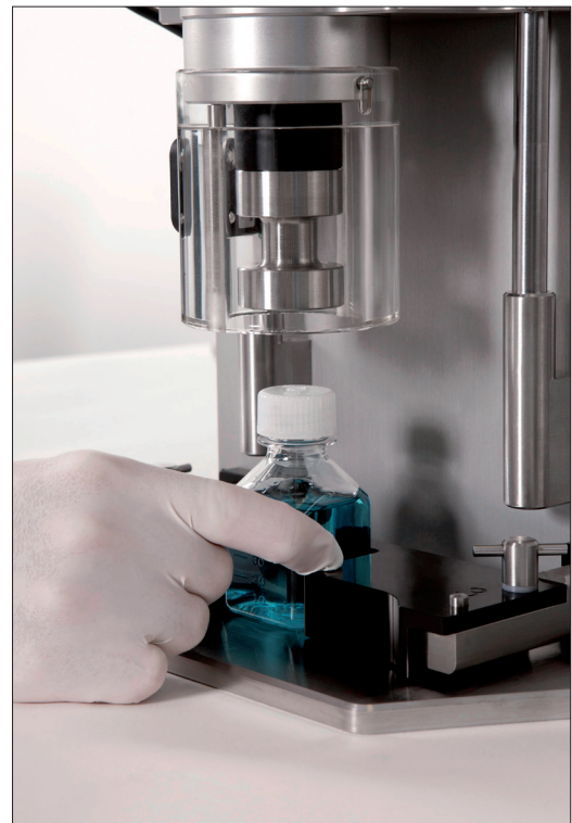
Customised format parts for bottles and screw caps. A changeover can be done in less than 5 minutes.
