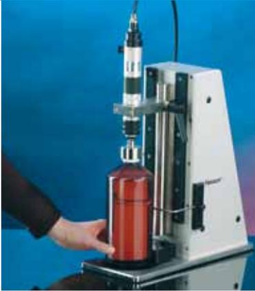
FC10 and FC32 are semi-automatic machines for tightening screw caps onto bottles.
