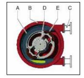
In phase 2 the product is drawn into the hose by the (continuous) turning motion of the rotor.
