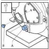
3. The pump housing can be filled with lubricant via the breather (A) on the cover. For this purpose remove the breather cap (B) and position a funnel (C) in the breather. Pour the lubricant in the pump housing via the funnel.
