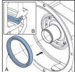
14. Check that the hub is clean and free of grease. Fit the bearings and the rings.
