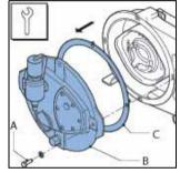
Put the hose pump on blocks. Make sure the space between the blocks is wide enough for the rotor to fall.
