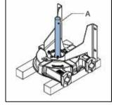
10. Dismount the circlip (A) with the correct tool.
