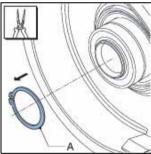
11. Dismount the bearings (A) with the correct tool, the spacer ring (B) and the retaining ring (C).
