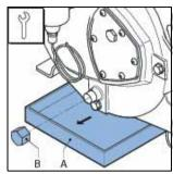
Position the drain plug (A) and tighten it firmly. For DuCoNite<sup>®</sup> 15 and DuCoNite<sup>®</sup> 20, remove the breather plug (B) before filling the lubricant. The DuCoNite<sup>®</sup> 10 can be filled without deaerating.
