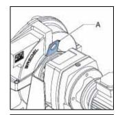
The complete hose pump, i.e. pump head, gearbox and electric motor, must be lifted using the lifting eye plus additional support using suitably rated straps or slings (A). For the weights, refer to § 10.1.6.
