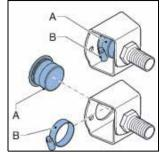
6. First fit the inlet port. Slide the rubber bush (D) over the hose. Push the bracket (A) and the hose clamp (B) over the hose together. Align the holes in the bracket with the ones at the front of the port. Position the two retaining bolts (C) and tighten them. Make sure the bolts are tightened with the correct torque. Refer to § 10.1.7.
