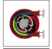
In phase 3, the second pressing shoe will subsequently compress the pump hose. Due to the continuous rotating movement of the rotor not only new product is sucked in, but also the already present product is pressed out by the pressing shoe. When the first pressing shoe runs from the pump hose, the second pressing shoe has already closed the pump hose and the product is prevented from flowing back. This method of liquid displacement is also known as the "positive displacement principle".
