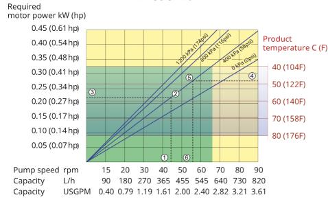
Note: The area of continuous operation diminishes with increased product temperatures. For product temperatures >40C, the area of continuous operation reduces to the corresponding red temperature line.
