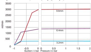
Sta-Pure element, 0-2 bar (0-30psi), 200rpm, counter-clockwise rotation
