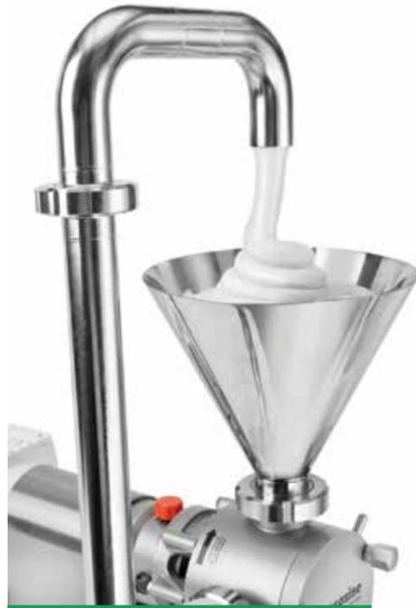
Put simply, if a production or process plant changes to a higher viscosity product, the impact on a sine pump is minimal is not negligible. For instance, using the same application parameters as before, but switching from a 20,000cP product to a 200,000cP product, the VHP of a sine pump increases by around 0.1, to 0.3VHP (0.22kW).
