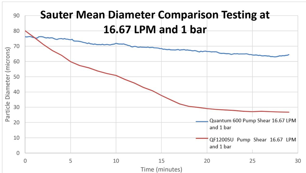
As shown by Graphs 1 and 2, the pump tested exhibited a defined rate or slope of decay in the Sauter mean diameter of the emulsion droplets. By evaluating the decrease in diameter, it is evident that under the same operating conditions this pump shows its own decay profile. While it is understood that droplet size and distribution will have an effect on the rate of decay as larger drops become smaller, the rate of the decay should diminish as the pump reaches the maximal shear zone.
