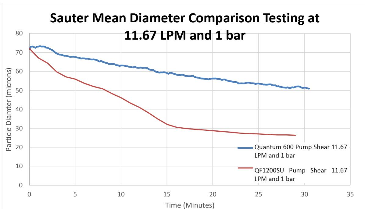
**Graph 2:** Watson-Marlow Quantum and Quattroflow QF1200SU pumps Sauter Mean Diameter shear testing at 16.67 LPM and 1 bar
