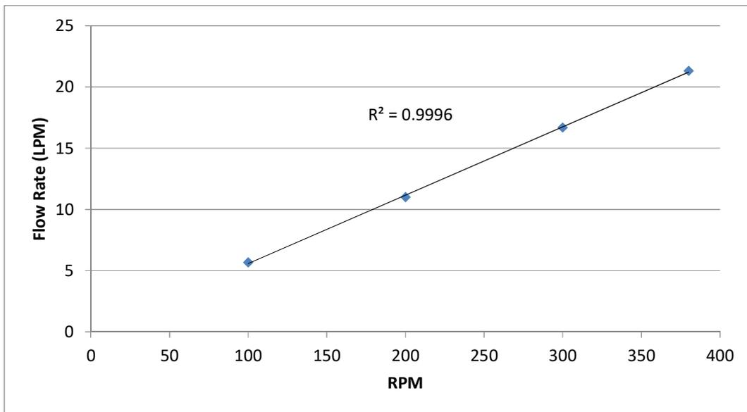
**Graph 7:** Watson-Marlow Quantum Pump difference in flow rate at various flow rates and pressures
