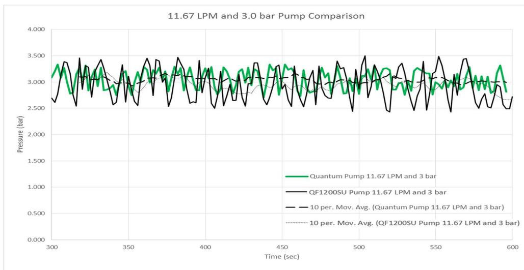
For both flow rates, the pulsation increases with pressure. There is greater pulsation at 11.67 LPM over 20 LPM. Appendix 1 has the Pulse Data Summary detailed results across the Watson-Marlow Quantum 600 pump and Quattroflow QF1200SU Pump at each set point.
