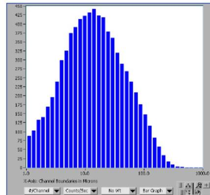
Thousands of Chord Lengths are measured each second to produce the Chord Length Distribution
