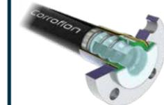
The PTFE liner in Corroflon has shallow convolutions which minimize the restriction in flow rates, and an external reinforcement wire in the external convolutions provides full vacuum resistance and kink resistance
