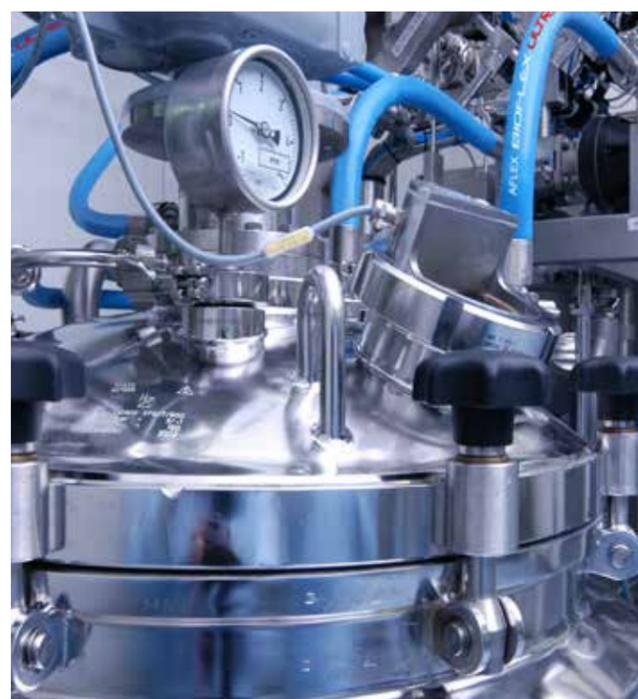
**Electrical continuity (EC)** is measured on assemblies only and between the metallic end fittings. EC assemblies are marked “M” grade and the electrical resistance between end fittings is less than 10<sup>2</sup>Ω (100Ω). The M-grade must be appropriate for the assembly construction. The following are not EC:
