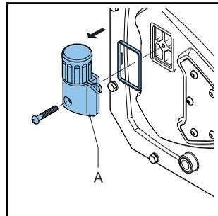
2. Mount the breather (A) with high-level float switch.
