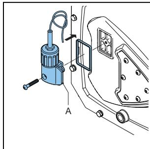
3. Connect the high-level float switch to the auxiliary power circuit via the 1.5 metre long PVC cable (2 x 0.34 mm<sup>2</sup>). Bear in mind that the electrical contact of the float switch is normally closed (NC). The knob is upwards for normally closed operation. When the lubricant level is (too) high the contact will open.
