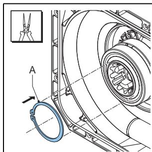
16. Fit the rotor (A). The rotor is placed on the bearings with a loose fit. Press the rotor on the hub until it clicks on the retaining ring.
