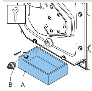
2. The pump housing can be filled with lubricant via the breather (A) on the cover. For this purpose remove the breather cap (B) and position a funnel (C) in the breather. Pour the lubricant into the pump housing through the funnel.
