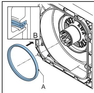
14. Slightly oil the inner ring of the (new) bearings and the seat on the hub. Fit the bearings and the rings. The bearings are placed on the hub with a slight interference fit. Use a pressing tool to press the bearings on the hub.
