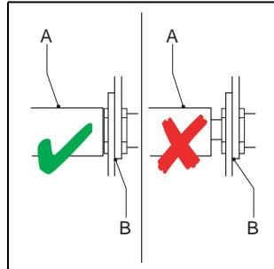
8. Place the hose clamp accurately on the track in the rubber bush. Tighten the bolt (B) of the hose clamp (A). Make sure the bolt is tightened to the correct torque. Refer to § 11.1.6.
