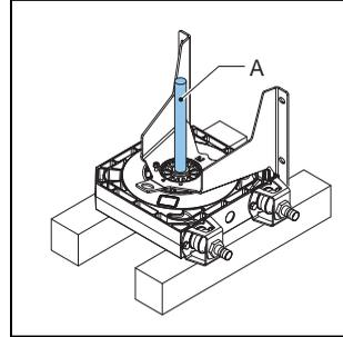
10. Dismount the circlip (A) with the correct tool.
