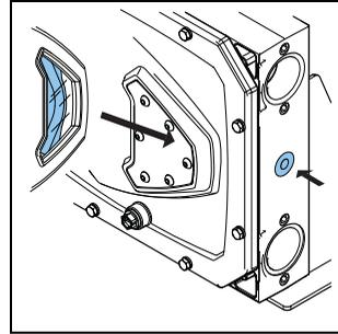
3. Remove the cover (B) by loosening the retaining bolts (A).
