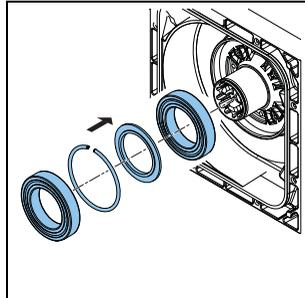
15. Mount the circlip (A).
