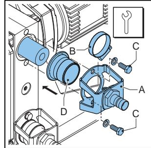
7. Turn the rotor in such a way that the hose (A) is pressed firmly against the bracket (B).
