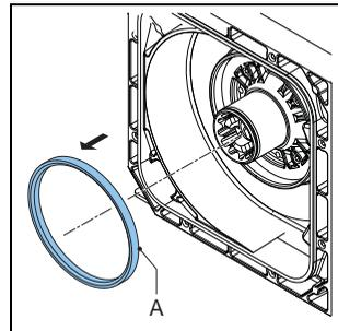
13. Fit a new seal ring (A) using good engineering practices. The seal ring must be fitted in the correct orientation (B). Make sure that the open side points to the pump cover.
