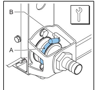
6. Loosen the bolts (A) of the bracket (B) and remove the bolts.
