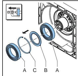
12. Remove the seal ring (A). Clean and degrease the bore. The holes in the pump housing can be used to drive out the old seal.
