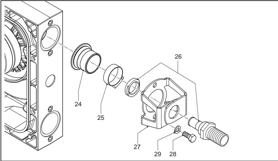
**i** All parts differ for the APEX10, APEX15 and APEX20 except for the bracket bolt and the bracket bolt washer.
