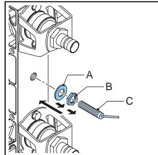
7. Tighten the nuts so that the distance between the sensor and the rotor (X) is between 0.75 mm and 1.25 mm.
