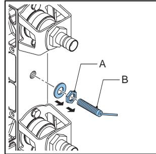
5. Mount the nut (B) and the sealing ring (A) on the new sensor (C).
