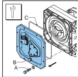
4. Remove the nut (A) and the old sensor (B).
