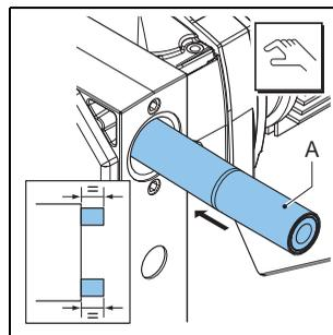
4. Check that the rubber bushes (A) are not deformed or damaged and replace them if necessary.
